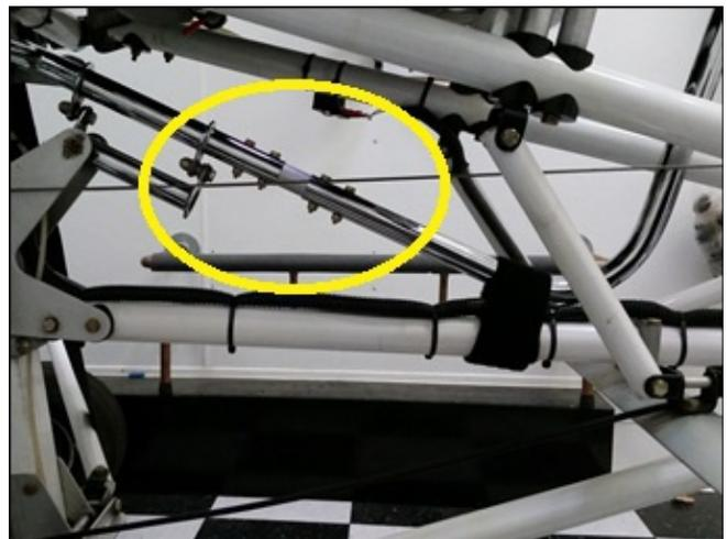
I finished the cyclic extension (in yellow circle, above) and got it installed. I used a piece of 6061-T6 solid round stock. The grip is now pretty close to the panel, but everything seems to be adjusted and working properly.
