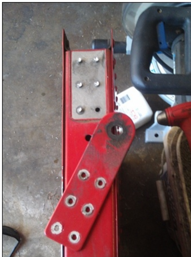
Above: Elongated holes in rudder mounting tab.
