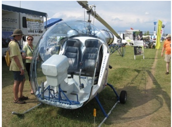
Carl Schneider brought his "Carlinator," (above,) a modified RFD Dominator powered by the HKS 700T turbocharged, two-cylinder engine, rated at 80 HP.
