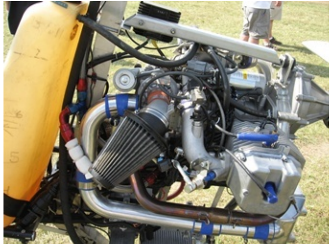
Carl Schneider brought his "Carlinator," (above,) a modified RFD Dominator powered by the HKS 700T turbocharged, two-cylinder engine, rated at 80 HP.
