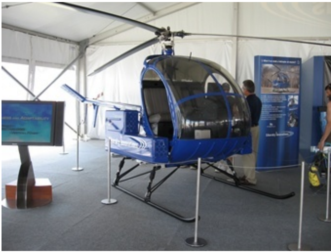
Sikorsky first displayed (above) its Firefly electric helicopter demonstrator at Oshkosh last year. The modified S-300C has a custom-built, 190-HP electric motor. The machine has not yet flown.
