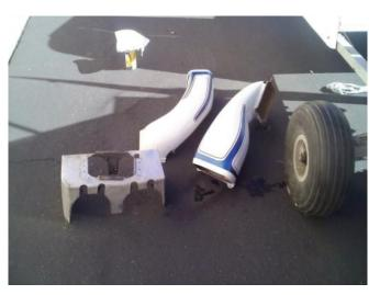
Above: Cooling shrouds removed during checkout of the Lycoming O-320 on the Hollmann. The engine shows good compression on all cylinders. Left: Dave Bacon with the Hollmann on a trailer. On the front cover: The Hollmann HA-2M as found. Only about a dozen Hollmann Sportsters were ever registered in the US, but the design proved influential, spawning imitators including the Marchetti, which used a similar frame design but without an enclosure.
