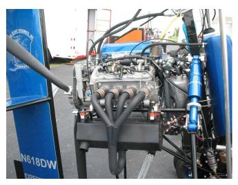
**Ernie Boyette of Rotor Flight Dynamics** is experimenting with the four-cylinder version of this engine, rated at 150 HP. This clean, blue, Dominator tandem has a custom-made muffler and airbox, and reportedly does a good job at quieting the raucous sled motor, which makes max HP at 10K RPM.
