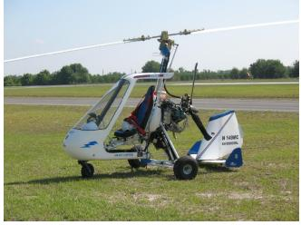
**Here's a rarity** - a <u>Sport Copter Vortex</u> on the east coast. Alex Bantum's machine (*above*) is powered by a 100 HP Rotax 912, an option which comes from Sport Copter with a steel mast and welded engine mounts. Alex is based in Port St. Lucie, FL.
