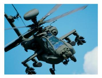
Noticeable differences from the Alpha model are wider base frame for more wiring and technology, exhaust curved vertical in back for rotors to dissipate heat better, sensor probes out both engines, and the radar dome on top of the rotors (*shown above*) for masting up over hiding spots to search for targets. Also the pilot night vision sensor above the target acquisition and designation system on the nose of the aircraft (*right*) is noticeably
