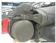
bigger. Only one in every group of Apaches need this radar dome, as the info picked up can be sent directly to the other Apaches. This dome tracks up to 276 targets, prioritizes them, and assigns them to the rest of the Apaches, which can then fire on those targets without ever being exposed.
