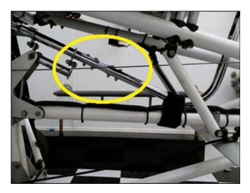
I finished the cyclic extension (in yellow circle, above) and got it installed. I used a piece of 6061-T6 solid round stock. The grip is now pretty close to the panel, but everything seems to be adjusted and working properly.
