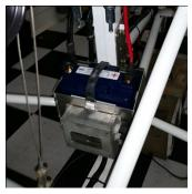
I got the custom battery box I ordered and got it installed. The battery I chose is a very small and light weight lithium battery with integral protection circuitry, so I don't need a special charger and it can be safely connected to a
