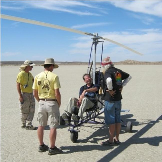
Above, a new design based on GyroBee geometry, but executed in welded thin-wall 4130 steel. William "Swani" Swanson (at right in above photo) talks with [CFI Mike Burton](#) (seated), who made the machine's maiden taxi tests at El Mirage. Below, a close-up of the unusual keel-to-main-gear bracing.
